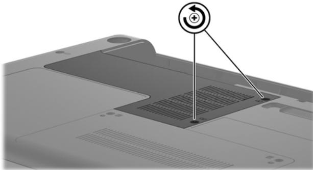
3. Lift cover off the computer. The mini-card compartment cover is included in the plastics kit, spare part number 600190-001.
