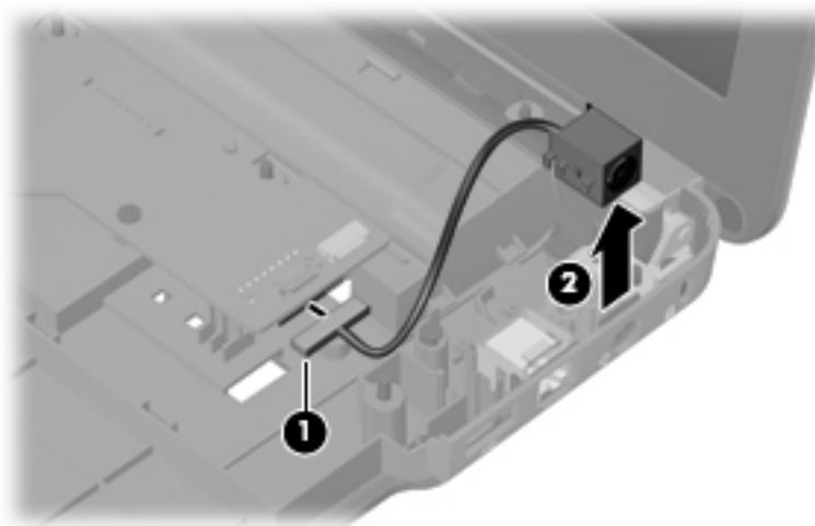
4. Remove the cable from the base enclosure.
