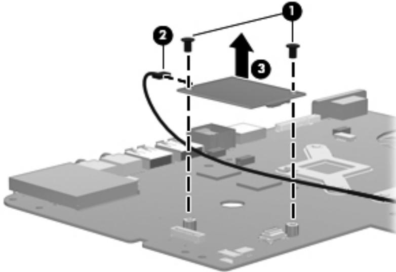
5. Remove the modem module.
