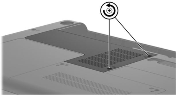
3. Lift the cover off the computer **(2)**. The mini-card compartment cover is included in the plastics kit, spare part number 600190-001.
