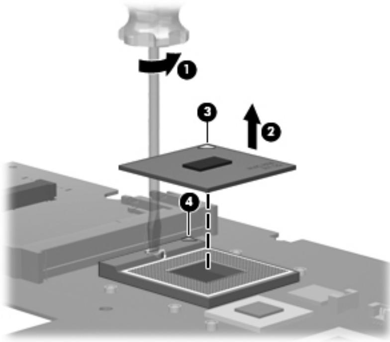
Reverse this procedure to install the processor.
