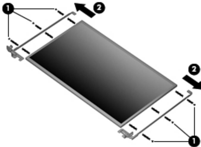
17. If it is necessary to replace the wireless antennas and cables, remove the adhesive strip **(1)** that secures each antenna to the display back cover.
