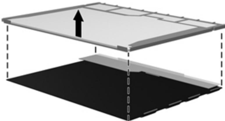
24. Recycle the LCD panel and backlight.
