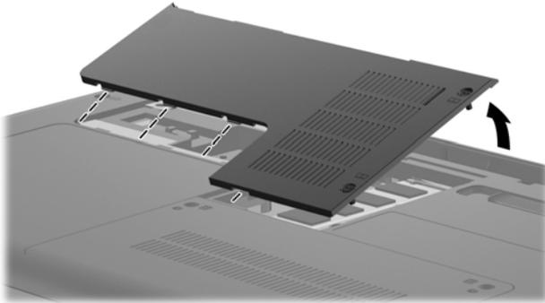
4. Spread the retaining tabs **(1)** on each side of the memory module slot to release the memory module. (The edge of the module opposite the slot rises away from the computer.)
