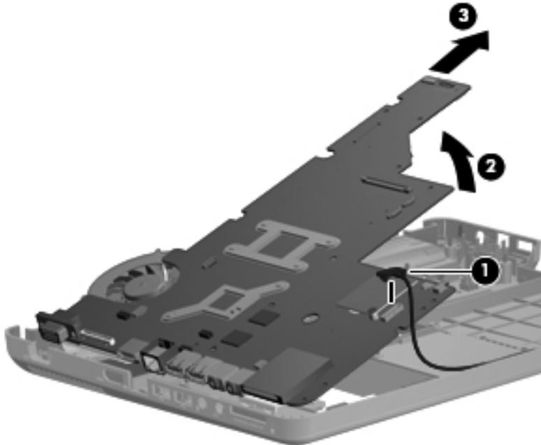
6. If it is necessary to replace the modem module cable, remove the RJ-11 connector (1) from the clip built into the base enclosure.
