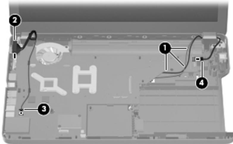
7. Remove the four black Phillips PM2.5×6.5 screws (1) that secure the display assembly to the computer.
