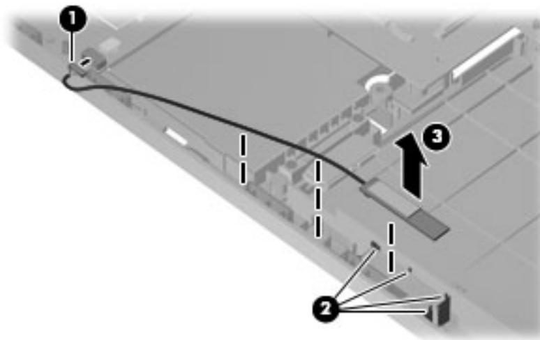
Reverse the above procedure to install the Bluetooth module.
